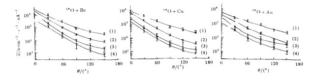
Fig.3 Emitted neutron angular distribution curves  $(1)E_n > 7 \text{ MeV}, (2) E_n > 11 \text{ MeV}, (3) E_n > 20 \text{ MeV}, (4) E_n > 50 \text{ MeV}$
