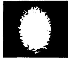
**Fig.2** CCD image of the synchrotron radiation from the bending magnet
