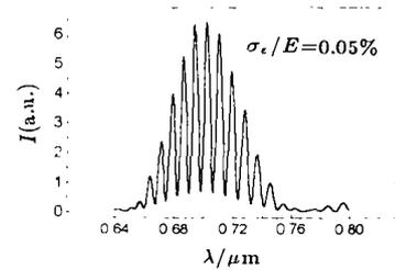
**Fig.6** Spontaneous emission for the TOK including only electron beam energy spread
