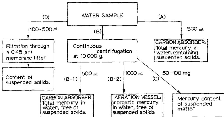
Fig.3 Mercury analysis procedure
