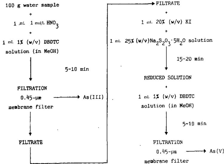
Fig.2 The optimized procedure for 100 mL samples runs as shown above. Loaded filters are dried over silicagel and packed in  $18 \times 9 \text{ mm}^2$  polythene containers equipped with iron flux monitors.
