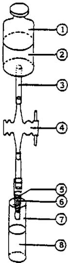
**Fig.1** The elution system for the  $\text{I}^-$ -  $\text{IO}_3^-$  separation and for the determination of  $\text{IO}_3^-$ , after Ref.[30]
