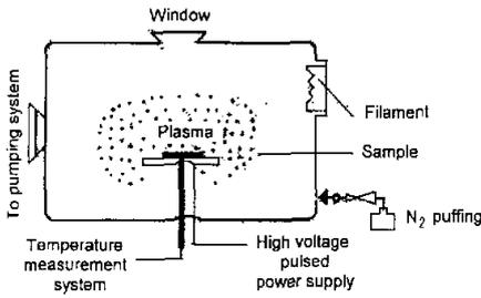
Fig.1 Schematic diagram of PSII-IBED system
