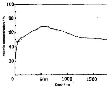
Fig.7 Nitrogen concentration profile of the sample implanted at temperature 600°C
