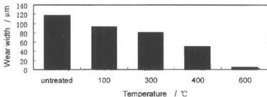
Fig.8 Width of the wear scar after 2000 revolutions of pin-on-disc wear test (25g load SiC pin)
