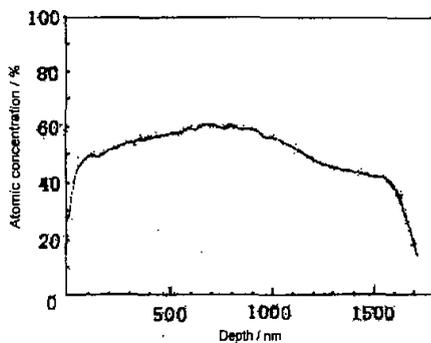
Fig.6 Nitrogen concentration profile of the sample implanted at temperature 400°C
