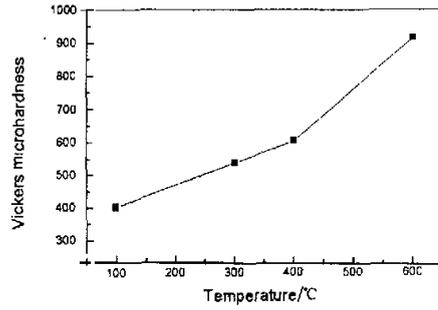
Fig.2 Microhardness as a function of temperature at load of 25 g
