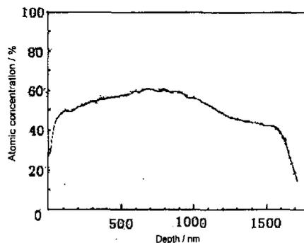
Fig.5 Nitrogen concentration profile of the sample implanted at temperature 300°C
