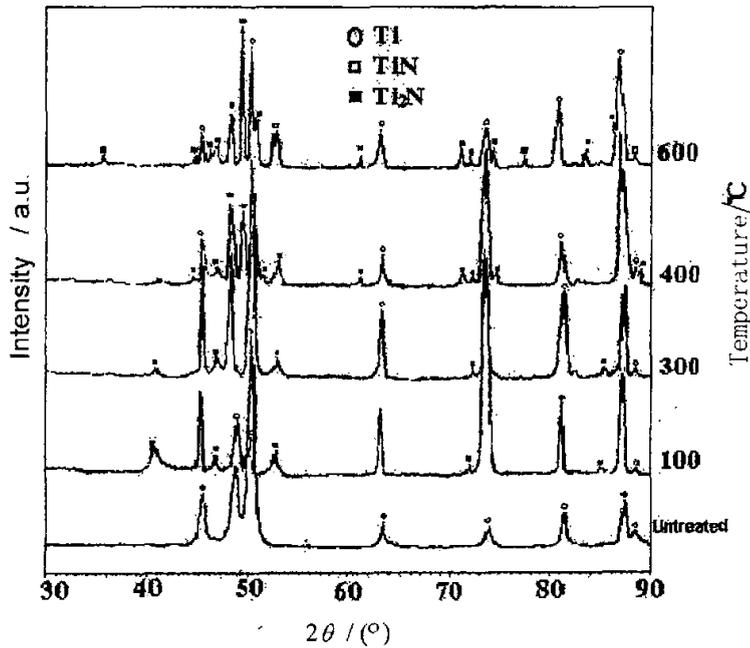
Fig.3 XRD patterns from the nitrogen-PSII-treated samples at different temperatures
