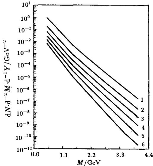
**Fig.1** The calculated dilepton spectra  $dN/dM^2dY$  for the evolution of the system in the phase diagram with the phase boundary at bag constant  $B^{1/4}=250$  MeV. Curves 1 to 6 denote, in turn, the spectra at rapidities  $Y=1.0, 1.5, 2.0, 2.5, 3.0$  and  $3.5$
