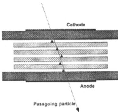
Fig.1 Cross section of a MRPC and the development of avalanche
