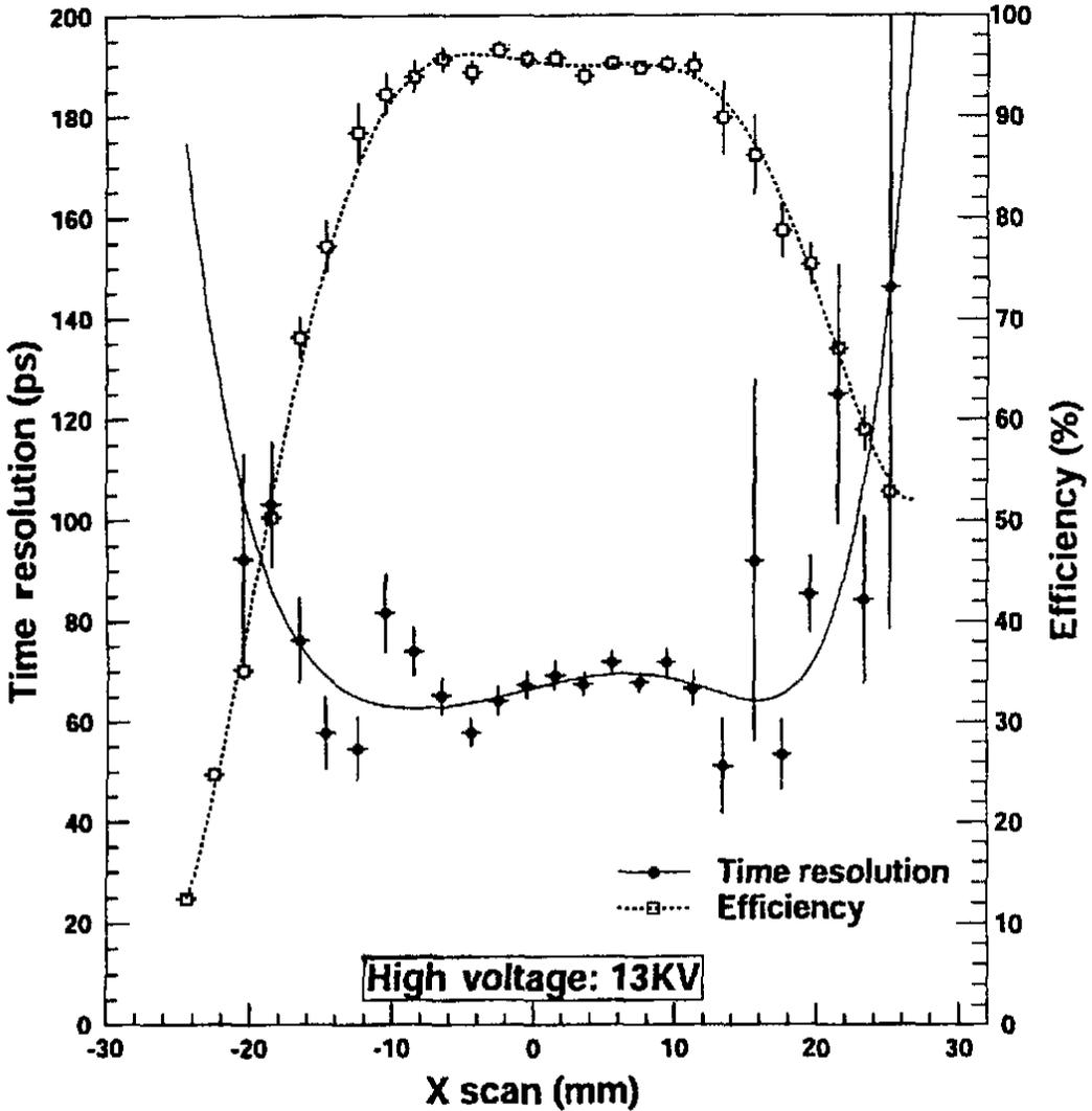
Fig.4 Scanning results of the MRPC at HV 13 kV
