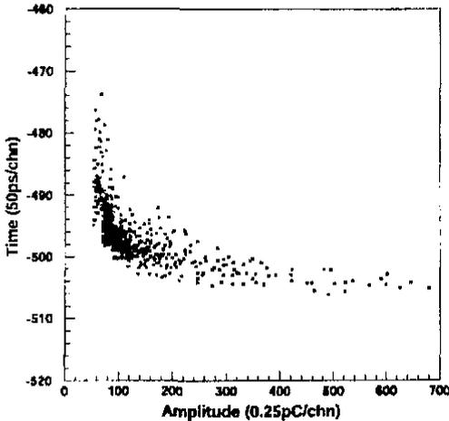
Fig.2 Time-amplitude relation of the signal from MRPC
