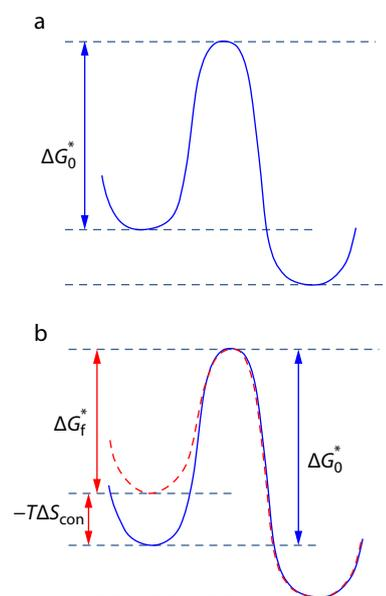
**Fig. 1** Schematic illustration of the free energy barrier of nucleation (a) at quiescent condition and (b) under flow from the conformational entropy reduction (CERM) model.  $\Delta G_0^*$  and  $\Delta G_f^*$  are the nucleation barrier at quiescent condition and under flow;  $\Delta S_{\text{con}}$  is the conformational entropy reduction of melt induced by flow.
