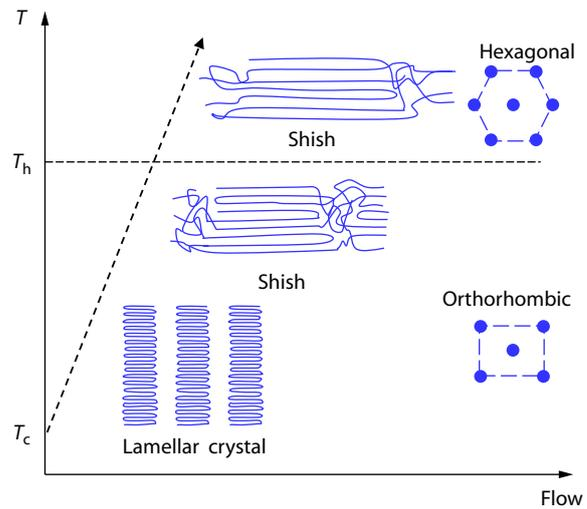
**Fig. 4** Schematic illustration of the crystal morphologies and structures of PE in the flow-temperature space.
